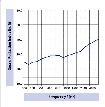
Test results for HALES SAWMILLS LTD - REFLECTIVE SOUND SCREEN, issued by: University of Salford (Acoustics Test Laboratory) UKAS accredited test laboratory No. 1262
