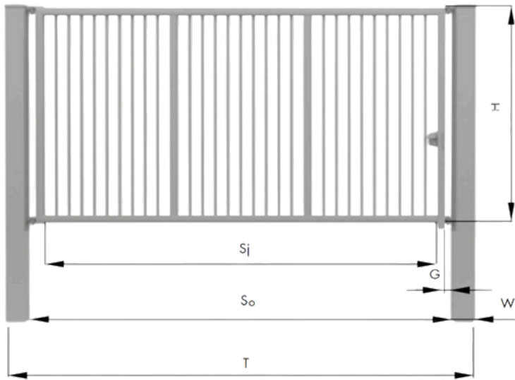
Fig. 35. Installation dimensions of the industrial single-leaf gate with designations.
