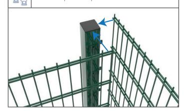
Attach the panels securely using the clamp bars and fixings provided with the fencing system. Inserting the M8 x 40 security bolts through the clamp bar and nylon spacer and into the rivnuts, do this for both sides of the corner post.
