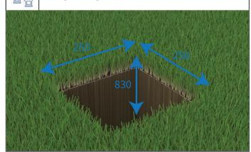
Place the post in the holes, ensure they're vertical and aligned to the fencing lines, then secure with concrete or post mix. Let them cure fully. Making sure the post cap is inserted before you dig in the post.
