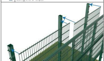
While holding the panels in position, attach the clamp bar using the M8 x 40 security bolts. Feed the bolts through the clamp bar, then through the nylon spacer and into each rivnut, starting from the top and working your way down.
