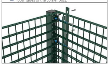
Finally, repeat these steps for all corners. Ensure both panels are securely fixed to the corner post, aligned correctly at 90 degrees, and level. Once all fixings are tightened and the structure is stable, clean the site and remove any excess materials or tools.
