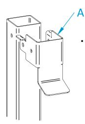
To Install the catch post sleeve assembly Firstly line the holes up in part A to the holes in the 80x80 post.
