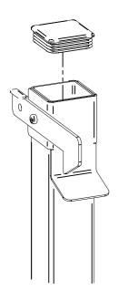
Now that the sleeve assembly is securely fitted the plastic insert can be fitted.
