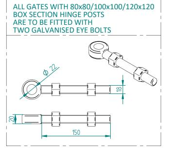
Component Name Quantity MESH-SLI-2042 - 868 MESH GATE SLIDER 2.0m X 2.5m WIDE MESH-HIN-2022 - 2.0m HIGH DIG IN MESH HINGE GATE POST 100X100 BOX SECTION ACCS-GEN-0001 - ADJUSTABLE GATE EYE BZP 130-150mm CW 20 ACCS-GEN-0101 - UNIVERSAL GATE DROP BOLT 2 ACCS-RIB-0003 - 60x60 BLACK RIBBED INSERTS ACCS-RIB-0006 - 100X100 BLACK RIBBED INSERTS
