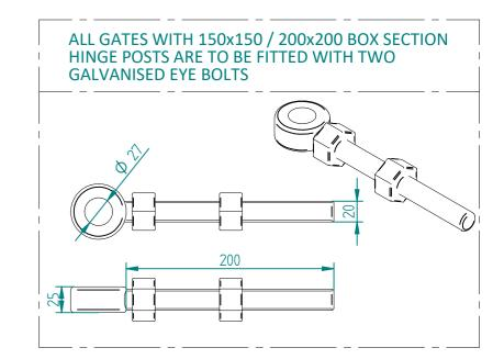
Item | Component Name Quantity ACCS-GEN-0002 - ADJUSTABLE GATE EYE G 200mm cw 25mm MESH-HIN-1872 - 1.8m HIGH BOLT DOWN MESH HINGE GATE POST 200X200 BOX SECTION D | MESH-REC-1832 - 1.8m HIGH BOLT DOWN MESH CATCH GATE POST 100X100 BOX SECTION ACCS-GEN-0101 - UNIVERSAL GATE DROP BOLT ACCS-RIB-0003 - 60x60 BLACK RIBBED INSERTS ACCS-RIB-0006 - 100X100 BLACK RIBBED INSERTS ACCS-RIB-0008 - 200x200 BLACK RIBBED INSERTS
