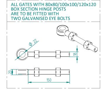
ItemComponent NameQuantityAMESH-SLI-1852 - 868 MESH GATE SLIDER 1.8m X 3.0m WIDE1BACCS-GEN-0001 - ADJUSTABLE GATE EYE BZP 130-150mm CW 202CMESH-HIN-1838 - 1.8m HIGH BOLT DOWN MESH HINGE GATE POST 120X120 BOX SECTION1DMESH-REC-1822 - 1.8m HIGH BOLT DOWN MESH CATCH GATE POST 80X80 BOX SECTION1EACCS-GEN-0101 - UNIVERSAL GATE DROP BOLT1FACCS-RIB-0003 - 60x60 BLACK RIBBED INSERTS2GACCS-RIB-0005 - 80x80 BLACK RIBBED INSERTS1HACCS-RIB-0020 - 120x120 BLACK RIBBED INSERT1
